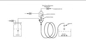
**Figure 5:** Bioreactor design. The anion droplets were introduced into the microgravity reactor. The polyanion droplets were moving together with polycation stream without any relative motion. The spherical capsules formed with uniform membrane thick less and pores diameter.
