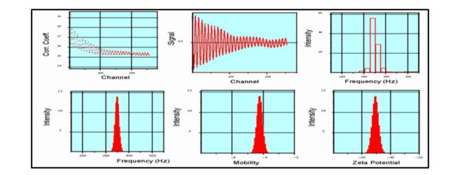
Figure 7: Stages of signal processing from the correlation function to a Fourier Transform analysis (FFT) to frequency, mobility and zeta potential spectrum.
