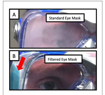
**Figure 1:** Photograph of (A) Standard Eye Mask (SEM) and (B) Filtered Eye Mask (FEM) [10]. Note that the amount of fog build up with the FEM is significantly lower than the SEM.
