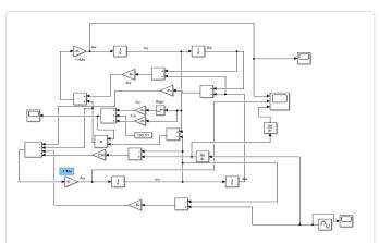
**Figure 5:** Simulink modeling of semi-active suspension system using Bingham model.
