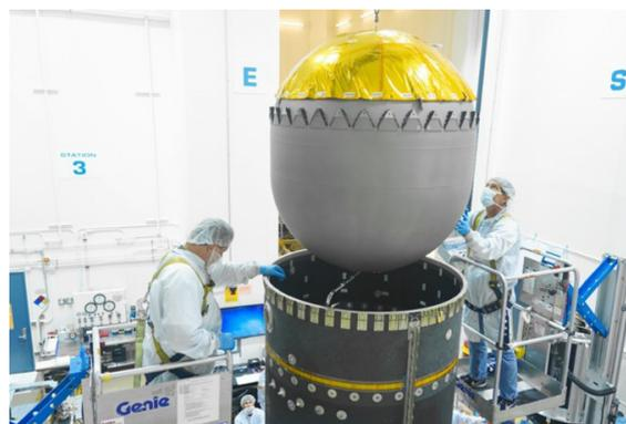
Figure 8: One bipropellant fuel tank being installed inside the main cylinder of OSAM 1 [21].
