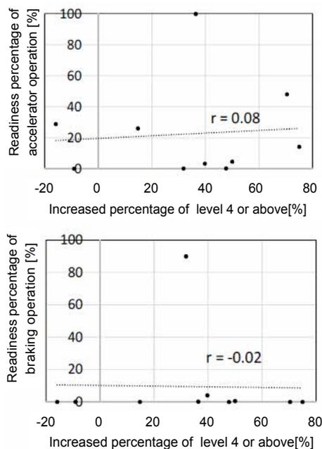
Figure 7: Relationship between the increase of sleepiness level and accelerator/brake readiness rate.
