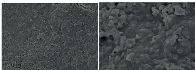
**Figure 14:** SEM micrographs of S/Z=0.3 with Cu solution (1000X - 5000X) [15].
