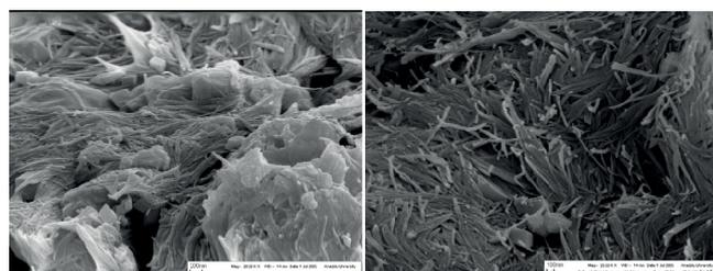
**Figure 17:** SEM micrographs of S/Z=0.3 with Cr solution (20000X - 25000X) [15].
