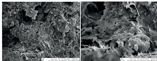
**Figure 16:** SEM micrographs of S/Z=0.3 with Cr solution (1000X - 5000X) [15].
