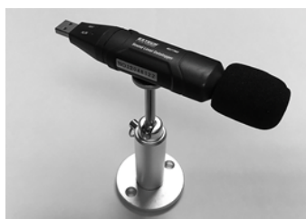
Figure 3: Extech Instruments USB Sound Level Datalogger with stand and windscreen used for SPL measurements.
