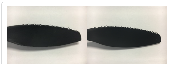
Figure 2: Propeller modifications with leading edge comb tip- and hub-oriented.
