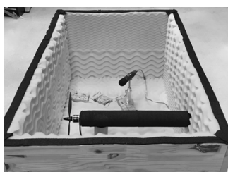
Figure 4: Sound chamber with electric motor, propeller, and sound datalogger installed.
