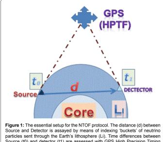
Source (t0) and detector (t1) are assessed with GPS High Precision Timing Facility (HPTF) [3]. The speed of neutrinos is taken at the speed of light. (Not to scale)
