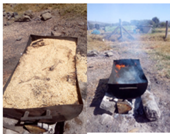
Figure 3: Carbonization of Sawdust & Water Hyacinth.
