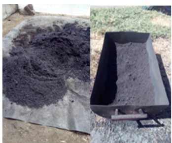
Figure 4: Carbonized Sawdust & Water Hyacinth.
