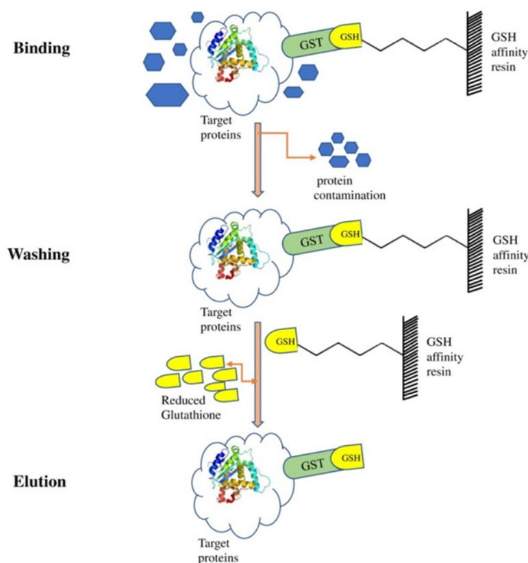
**Figure 2:** A Diagrammatic demonstration of Glutathione Affinity chromatography. Cleared lysate which carried GST fusion proteins that attach to immobilized glutathione (GSH, Bind). Non-binding proteins are discharge (washed) from the resin (Wash) and by the addition of excess reduced glutathione bound GST fusion proteins are eluted (Elute).
