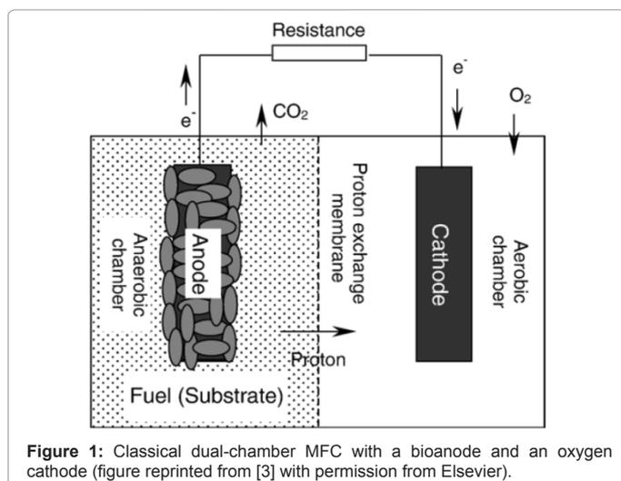
**Figure 1:** Classical dual-chamber MFC with a bioanode and an oxygen cathode (figure reprinted from [3] with permission from Elsevier).
