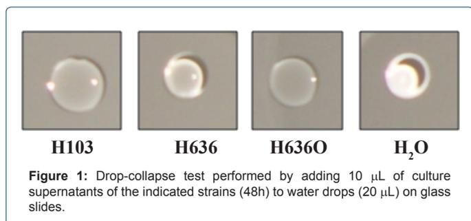
**Figure 1:** Drop-collapse test performed by adding 10 µL of culture supernatants of the indicated strains (48h) to water drops (20 µL) on glass slides.
