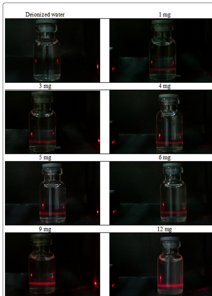
Figure 1: The Faraday-Tyndall effect observation on BSA-loaded nanoemulsion with different BSA concentrations. The red beam width easily indicated the particle size of oil globules.
