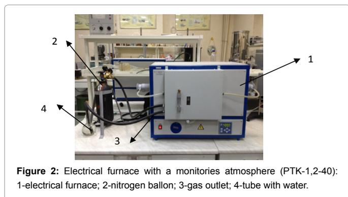
Figure 2: Electrical furnace with a monitored atmosphere (PTK-1,2-40): 1-electrical furnace; 2-nitrogen ballon; 3-gas outlet; 4-tube with water.
