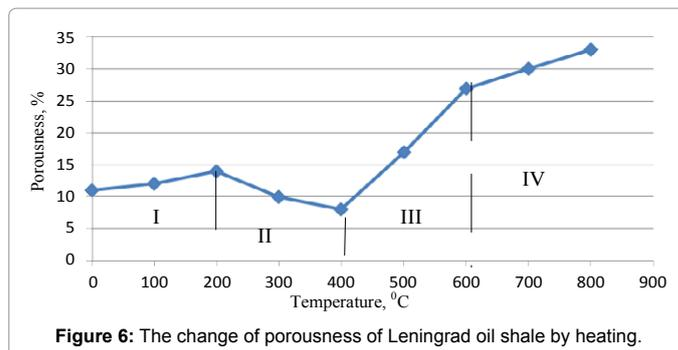
Figure 6: The change of porousness of Leningrad oil shale by heating.
