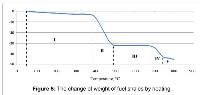
Figure 5: The change of weight of fuel shales by heating.
