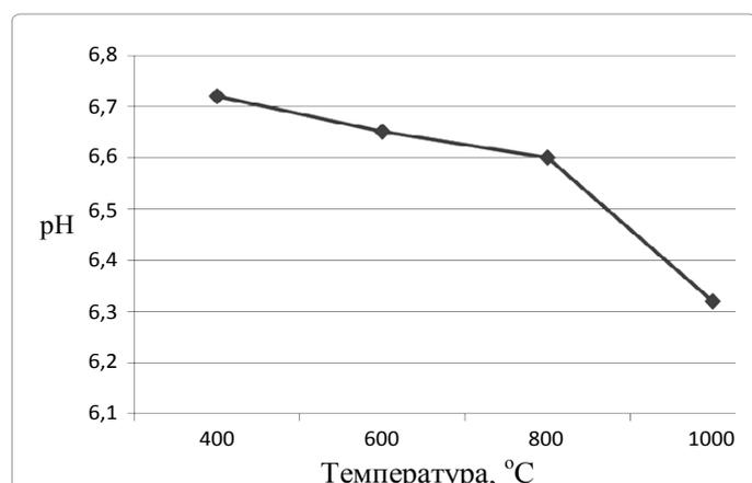
Figure 7: The influence of temperature of heat treatment on a change in pH of water sphere.
