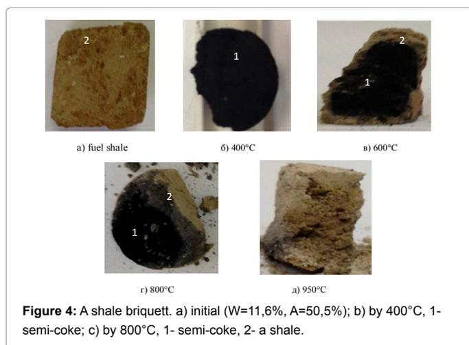
Figure 4: A shale briquet. a) initial (W=11,6%, A=50,5%); b) by 400°C, 1- semi-coke; c) by 800°C, 1- semi-coke, 2- a shale.
