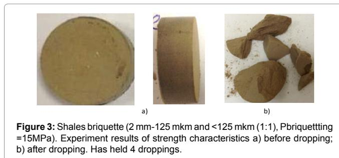
Figure 3: Shales briquette (2 mm-125 mkm and <125 mkm (1:1), P briquetting = 15MPa). Experiment results of strength characteristics a) before dropping; b) after dropping. Has held 4 droppings.
