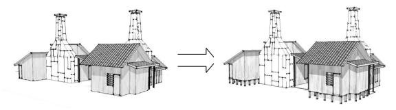
Fig. 13. Applying knock down semi-raised platform house model to avoid mud and humid floor.
