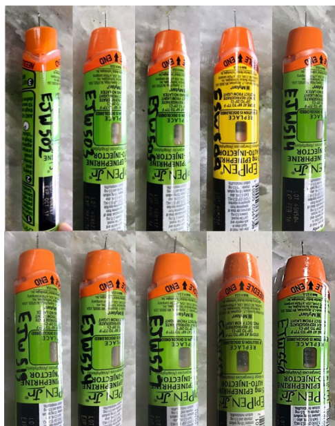
Figure 3: Washed EpiPen and EpiPen Jr. devices that didn't release the orange needle shroud after they were triggered, leaving exposed needles.
