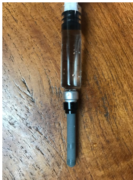
Figure 4: A washed EpiPen with visible drops of liquid beneath the clear plastic housing.
