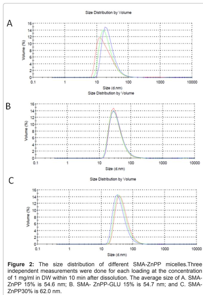
Figure 2: The size distribution of different SMA-ZnPP micelles. Three independent measurements were done for each loading at the concentration of 1 mg/ml in DW within 10 min after dissolution. The average size of A. SMA-ZnPP 15% is 54.6 nm; B. SMA-ZnPP-GLU 15% is 54.7 nm; and C. SMA-ZnPP 30% is 62.0 nm.
