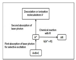
Fig. 1 General scheme of the chemical separation by laser radiation excitation [5].
