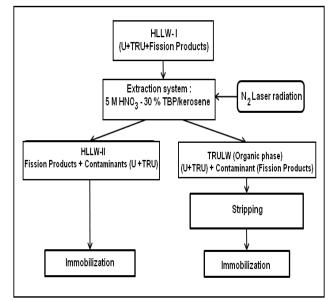
Fig. 4 Adaptation of HLLW treatment process technology generated from RPI or RMI through the extraction process with solution system of 5 M HNO<sub>3</sub> -30% TBP / kerosene using  $N_2$  laser pulse radiation.
