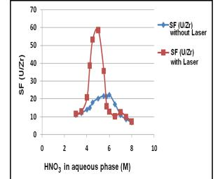
Fig. 3 Effect of  $N_2$  Laser pulse radiation on SF <sub>(U/Zr)</sub> in extraction system of HNO<sub>3</sub>-30% TBP/Kerosene (iradiation of laser for 90 minutes at voltage 100 volts) [18].
