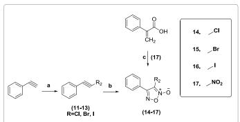
Figure 2: (b) NaNO<sub>2</sub>, H<sub>2</sub>SO<sub>4</sub>,DME, -5C, rt, overnight, 29-30%; (c) NaNO<sub>2</sub>, H<sub>2</sub>SO<sub>4</sub>, DCE, 50°C, 1h, 71%.
