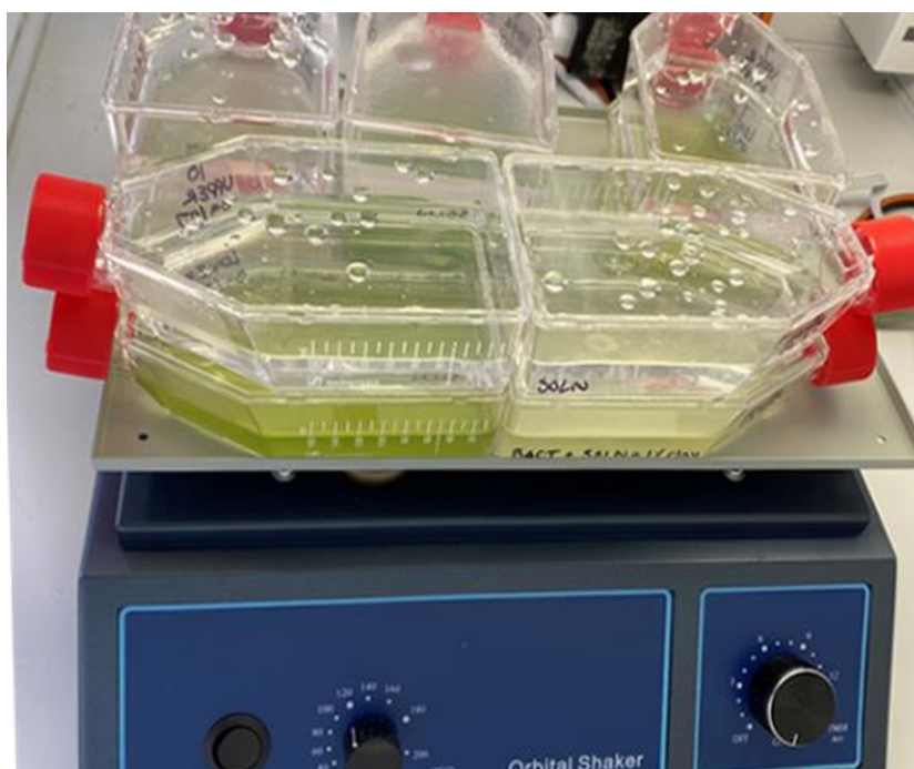
Figure 1: Experimental set-up. M. aeruginosa cells were grown in three growth solutions' described in Table 1 in the lower flasks. Flasks filled with solutions with and without clay were placed on top of the lower flasks to create identical light conditions for all cases. The flasks were placed on a shaker set to 110 rpm within an incubator with white fluorescent light illuminating from the top of the flasks at 12 h:12h light/dark cycle.
