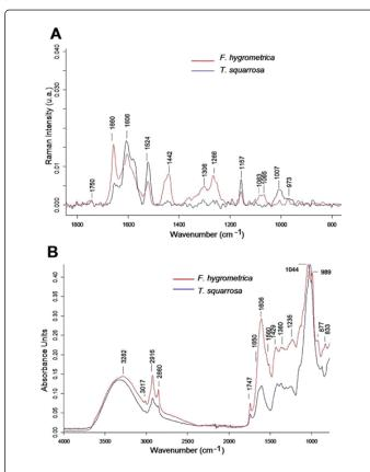
**Figure 5:** Comparative vibrational spectroscopy between desiccated gametophytes of *T. squarrosa vs.* spores of *F. hygrometrica* (A) FT-Raman spectra (B) FT-IR spectra.
