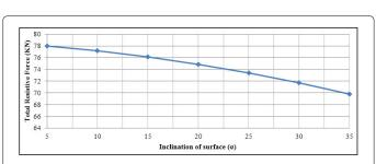
Figure 9: Effect of surface inclination on total resistive force.
