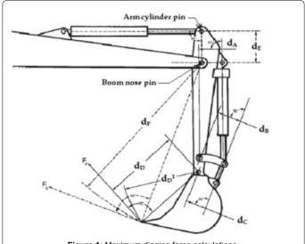
Figure 1: Maximum digging force calculations.
