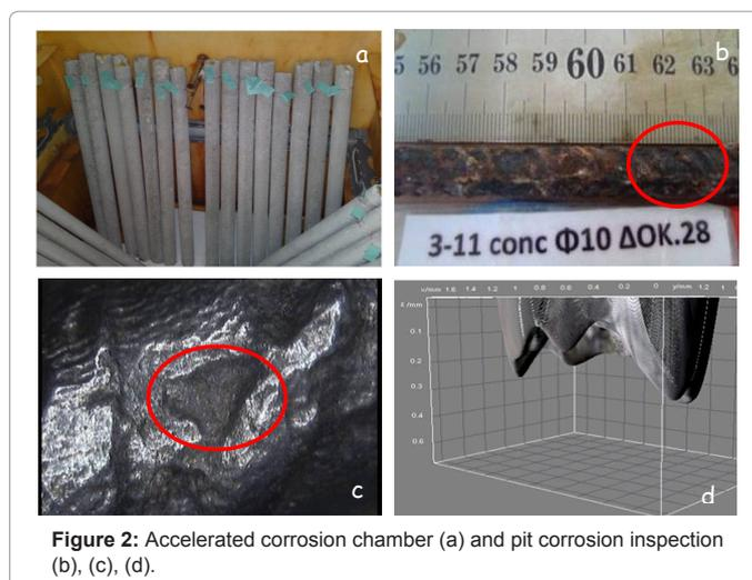
Figure 2: Accelerated corrosion chamber (a) and pit corrosion inspection (b), (c), (d).
