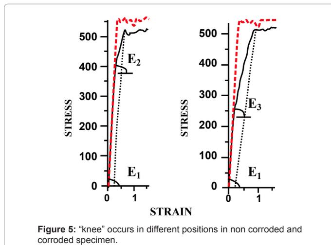
Figure 5: “knee” occurs in different positions in non corroded and corroded specimen.
