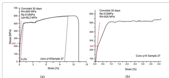
Figure 4: Indicated stress-strain diagram of a corroded steel bar.
