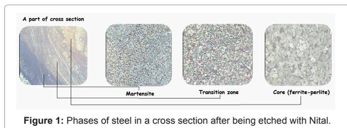
Figure 1: Phases of steel in a cross section after being etched with Nital.
