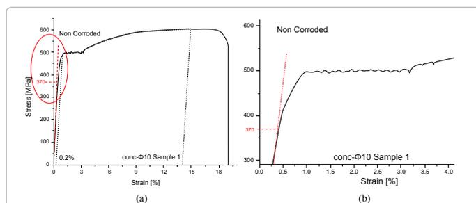
Figure 3: Indicated stress-strain diagram of non corroded steel bar.
