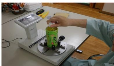
**Figure 1:** The equipment used and measurement position. Digital Torque Meter 2TME450CN (N-cm), c, Co., Ltd.
