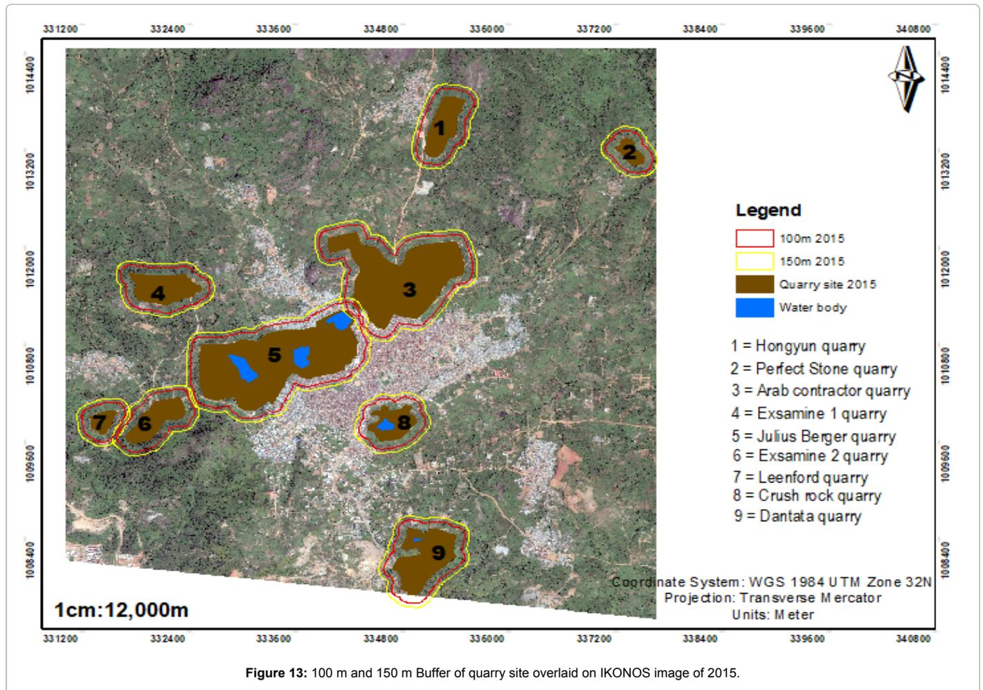
Figure 13: 100 m and 150 m Buffer of quarry site overlaid on IKONOS image of 2015.
