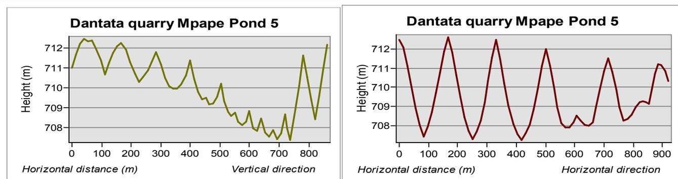
Figure 12: The depth profile of pond 5 within Dantata quarry site. Source: Fieldwork (2017).
