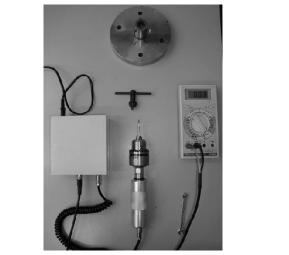
Figure 3: Torsiometer device and experimental set-up tools used for mechanical debonding test.
