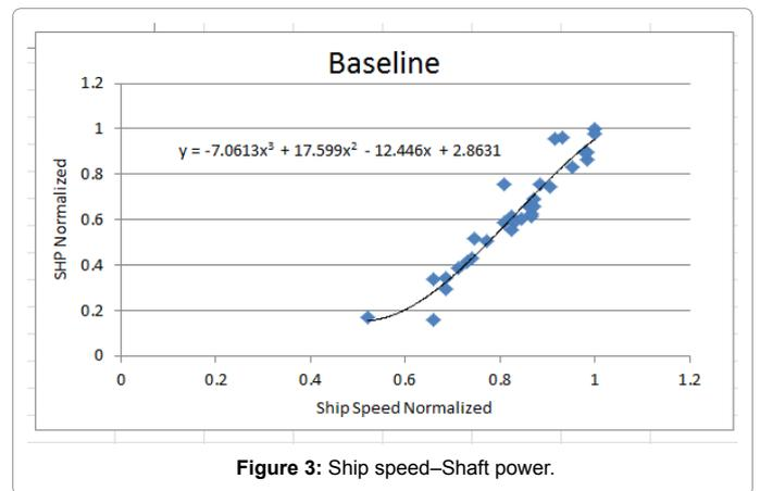
Figure 3: Ship speed–Shaft power.
