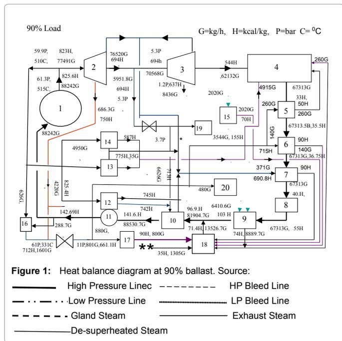
**Figure 1:** Heat balance diagram at 90% ballast. Source:
