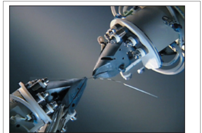
Figure 1: Bending orthodontic archwires into particular shape.
