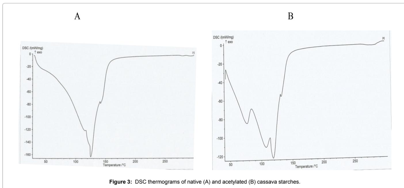
Figure 3: DSC thermograms of native (A) and acetylated (B) cassava starches.
