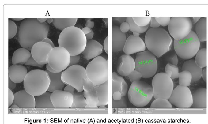
Figure 1: SEM of native (A) and acetylated (B) cassava starches.
