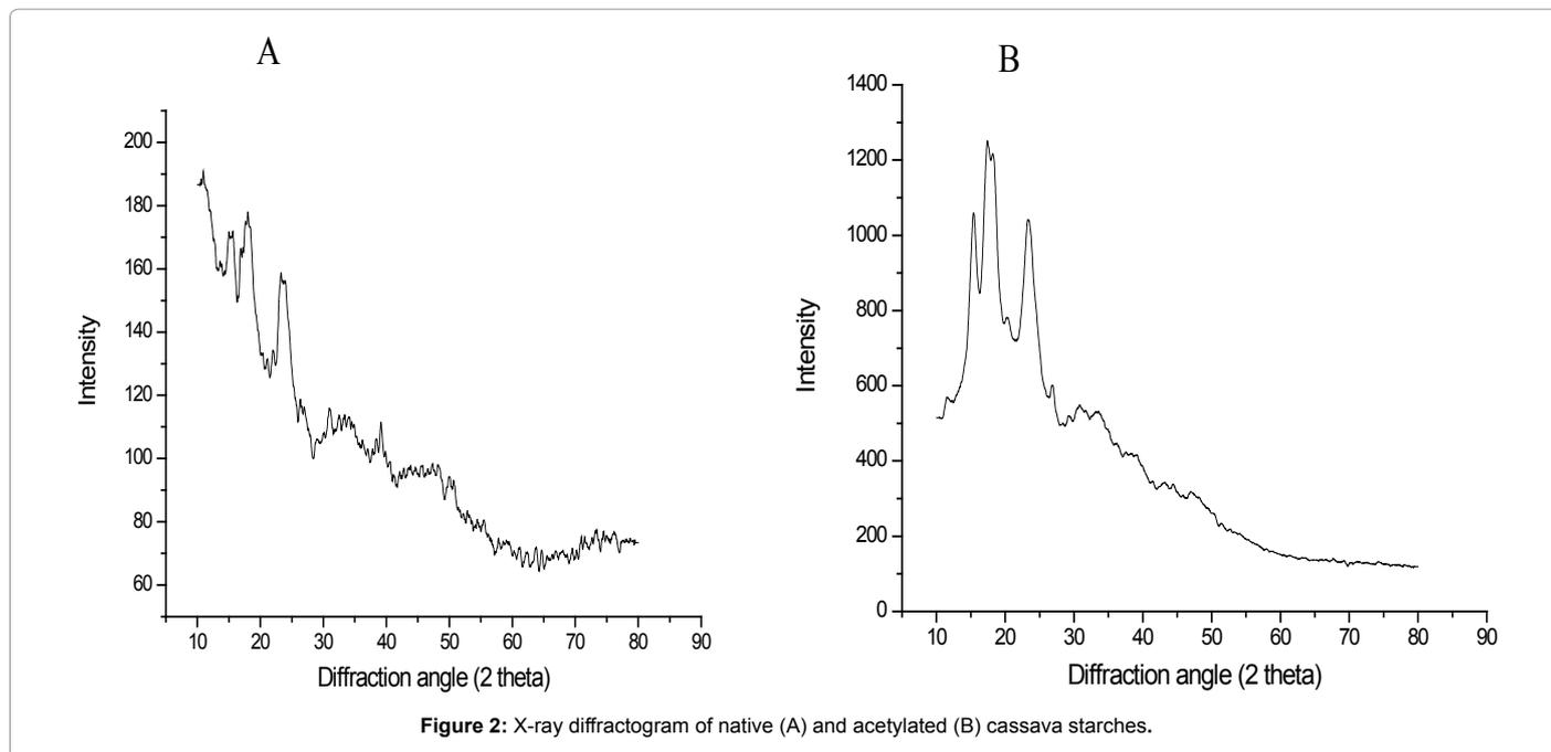
Figure 2: X-ray diffractogram of native (A) and acetylated (B) cassava starches.
