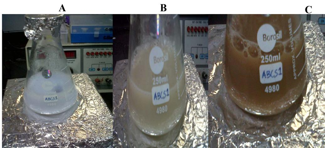
**Figure 6:** Stepwise preparation of Ag/drug/starch nanocomposites (A; starch suspension, B; starch suspension with drug/silver nitrate/NaBH<sub>4</sub> at 2 min, C; starch suspension with drug/silver nitrate/NaBH<sub>4</sub> at 15 min).
