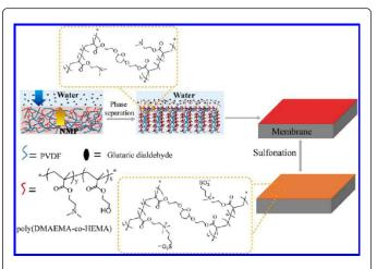
**Figure 2:** Schematic description of phase separation in the formation of zwitte rionic PVDF/PSH-blend membranes using random PDH copolymer as an additive, combined with *in situ* cross-linking and subsequent sulfonation, adopted from Zhu et al. [70].
