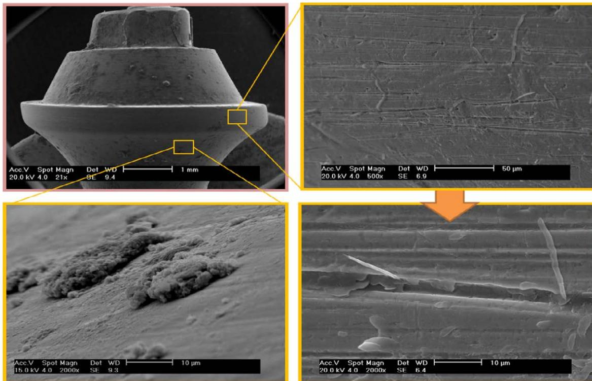
**Figure 1:** SEM micrograph of (A-D) commercial abutment surfaces covered with a multi-specie biofilm grown for (B-D) 72 h in BHI medium enriched with 5% sucrose, obtained by secondary electron (SE) mode at 15 kV.
