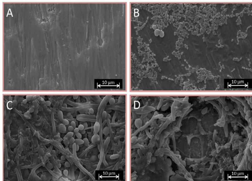
**Figure 3:** SEM micrograph of polished titanium surface (A) free of biofilms and covered with a multi-species biofilm grown for (B) 24, (C) 72 and (D) 96 h in BHI medium enriched with 5% sucrose, obtained by secondary electron (SE) mode at 15 kV.
