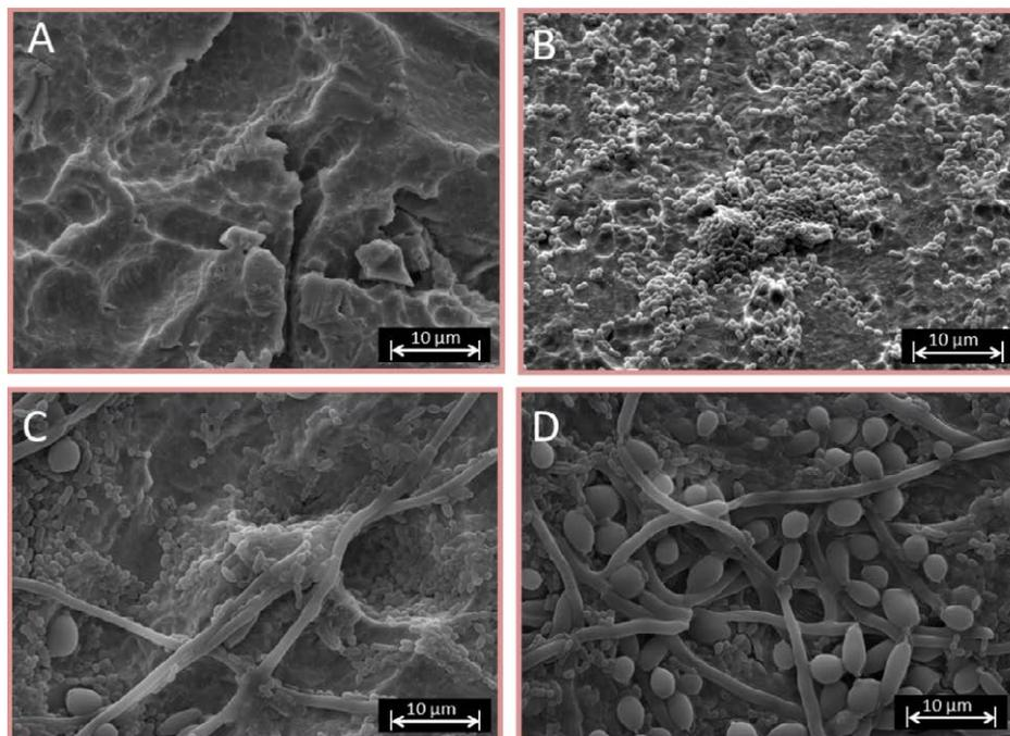
**Figure 4:** SEM micrograph of SLA titanium surface (A) free of biofilms and covered with a multi-specie biofilm grown for (B) 24, (C) 72 and (D) 96 h, obtained by secondary electrons (SE) mode at 15 kV.
