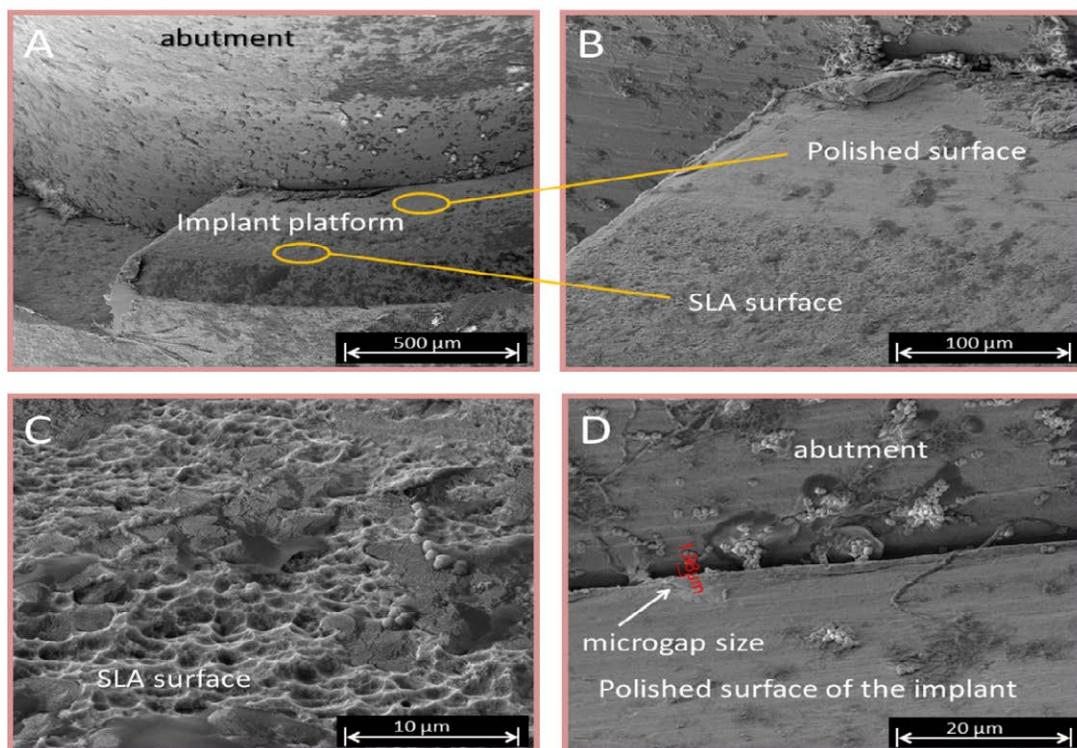
**Figure 2:** (A) SEM micrograph of commercial abutment-implant assembly. (B) Upper view of the platform revealing rough (SLA) and polished surfaces. (C) Topography of the commercial SLA surface covered with a multi-specie biofilm grown for 72 h in BHI medium with 5% sucrose. (D) Microgap size at the implant-abutment connection. SEM micrographs obtained by secondary electron (SE) mode at 15-20 kV.
