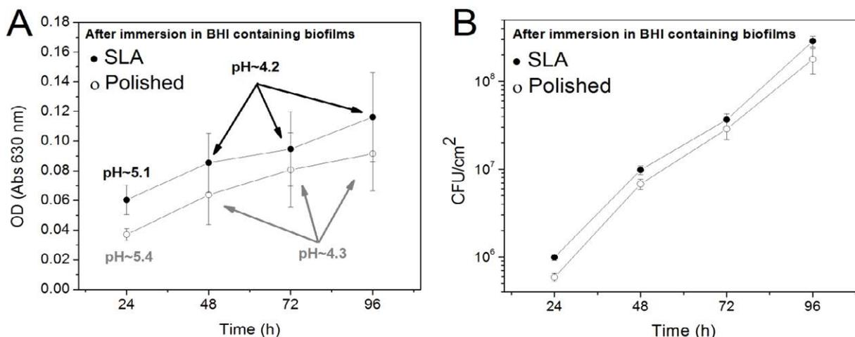
**Figure 5:** (A) Optical absorbance (Abs) expressing the development of multi-species biofilm biomass on polished and SLA surfaces. Also, the pH of the growth medium after 96 h in BHI medium enriched with 5% sucrose (37 C, 150 rpm). (B) Colony-forming unit (CFU) of multi-species biofilm biomass grown on polished and SLA surfaces for 96 h in BHI medium enriched with 5% sucrose (37 C, 150 rpm).
