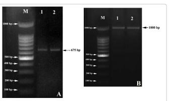
**Figure 1:** Agarose gel (2%) showing *Flavobacterium columnare* specific 16S rDNA gene fragment amplicons of primers (A): CoIF, CoIR and (B): CoI72F, CoI1260R. Lane M: 100 bp molecular weight DNA marker; Lane 1: RG1 - DNA isolated from the gill of *Labeo rohita*; Lane 2: C1 - DNA isolated from the muscle tissue of caudal peduncle region of *Ctenopharyngodon idella*.
