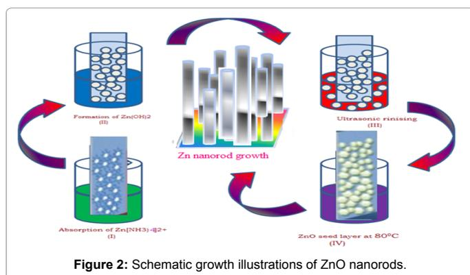
Figure 2: Schematic growth illustrations of ZnO nanorods.
