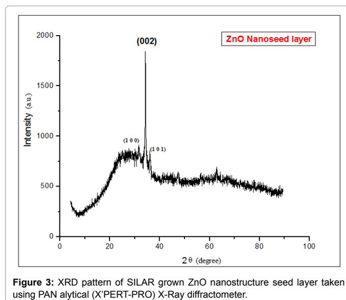
Figure 3: XRD pattern of SILAR grown ZnO nanostructure seed layer taken using PAN alytical (X'PERT-PRO) X-Ray diffractometer.
