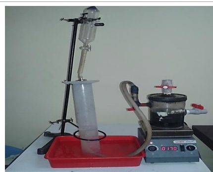
Figure 3: Batch type stirred tank reactor setup.
