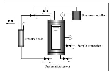
**Figure 1:** Apparatus for  $CO_2$  top pressure treatment. The preservation system with a sample connection, temperature monitor, pressure controller and pressure vessel placed in a thermostat keep a constant  $CO_2$  top pressure for shanlan rice wine preservation. The pressure controller play a pressure adjustment role and the pressure vessel act as a buffer to discharge the residual air in the main vessel.
