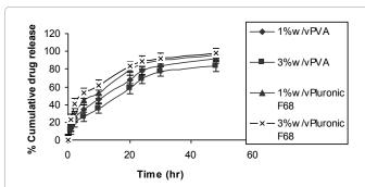
Figure 9: Drug release profile of lomustine from nanoparticles as a function of PVA and surfactant Pluronic F68 concentration.
