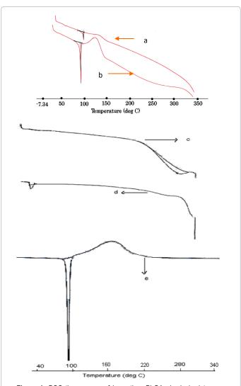
**Figure 1:** DSC thermogram of lomustine: PLGA physical mixture. a: endotherm of sample mixture 1:1 lomustine: PDLG 5002, b: endotherm of sample mixture 1:1 lomustine: PDLG 7502. c: polymer PDLG 5002, d: polymer 7502, e: lomustine.
