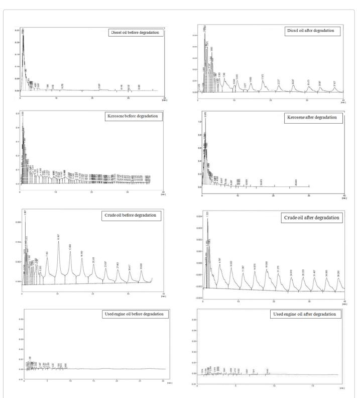
Figure 2: Figure showing GLC profiles of the diesel, kerosene, crude oil, and used engine oil before (control) and after (test) degradation (after 28 days of incubation) by the plasmid cured strain.
