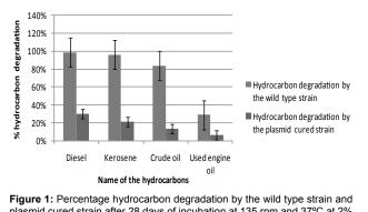
plasmid cured strain after 28 days of incubation at 135 rpm and 37°C at 2% ( $\nu/\nu$ ) substrate concentration (petroleum oil). Results are in mean  $\pm$  S.D., where n=3.
