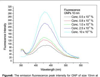
**Figure6:** The emission fluorescence peak intensity for GNP of size 10nm at different concentrations.
