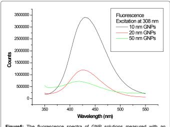
**Figure5:** The fluorescence spectra of GNP solutions measured with an excitation wavelength of 308 nm.
