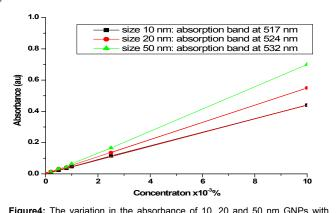
Figure4: The variation in the absorbance of 10, 20 and 50 nm GNPs with concentration.
