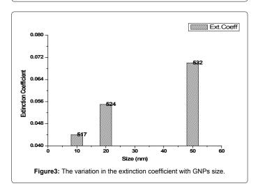
Figure 3 shows the variation in the extinction coefficient with GNPs size. When the GNP size changed from 10 nm to 50 nm, the maximum extinction of Surface Plasmon Band (SPB) shifted from 517 nm to 532 nm in the visible region which may be attributed to the surface plasmon oscillation of free electrons. The surface plasmon resonance of the gold particles is red shifted with increase in particle size in accordance with Mie theory [22].
