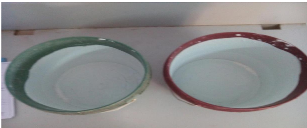
Figure.1. Paint commercial Calcium powder and commercial gum was mixed with PSB and painted on the inner surface of the buckets. The buckets were loaded with ¾ the volumes of different samples for bioleaching of fluoride where the concentration remained was determined by the spectrophotometric analysis at 542 nm.
