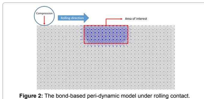
Figure 2: The bond-based peri-dynamic model under rolling contact.
