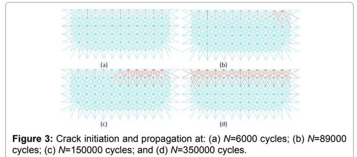
Figure 3: Crack initiation and propagation at: (a)  $N=6000$  cycles; (b)  $N=89000$  cycles; (c)  $N=150000$  cycles; and (d)  $N=350000$  cycles.
