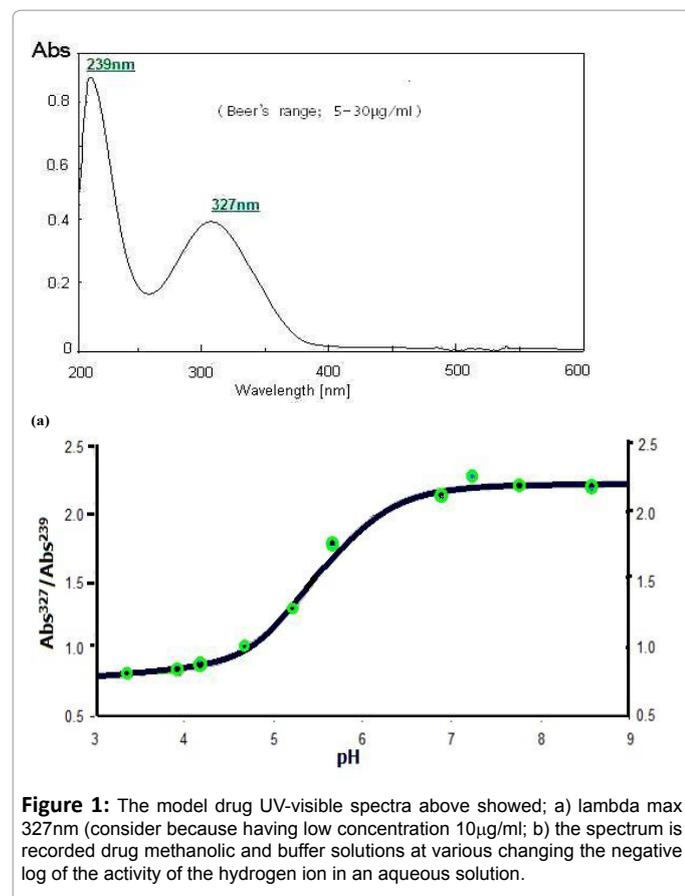
**Figure 1:** The model drug UV-visible spectra above showed; a) lambda max 327nm (consider because having low concentration 10µg/ml); b) the spectrum is recorded drug methanolic and buffer solutions at various changing the negative log of the activity of the hydrogen ion in an aqueous solution.
