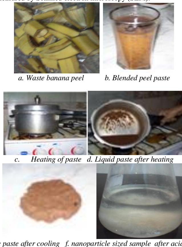
Figure 1. Photograph shows different steps of producing nano-particle from lignocellulose.
