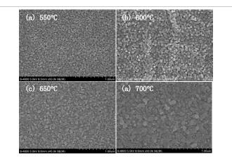
**Figure 3:** SEM images of the ZnO thin films annealed at (a) 550°C; (b) 600°C; (c)650°C; and (d) 700°C.
