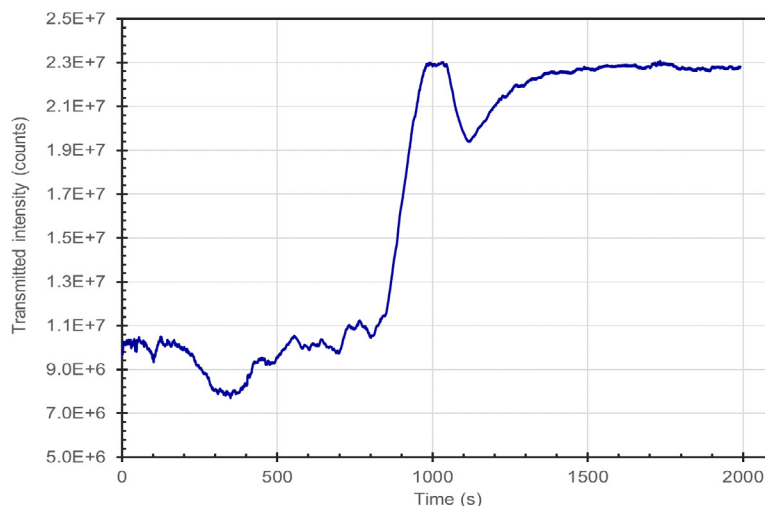
Figure 6: Drying kinetics of 2 mm Oligo-G solution in TE buffer applied to the NAM-PC nanosensor.
