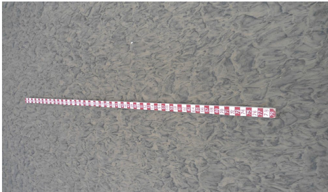
Plate 4: Current ripple marks aligned in the direction of flood tidal currents transport due north (left) at updrift foreshore.
