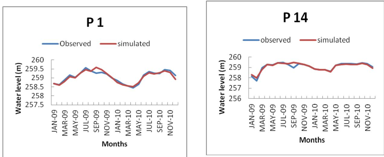
Figure 2: Observed versus Simulated head at the end of each stress period for piezometer 1 and 14
