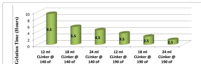
Figure 3: Temperature and crosslinker effect on gel time of water-shutoff for 2% KCl.
