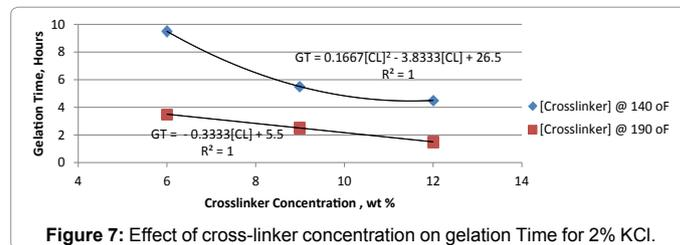
Figure 7: Effect of cross-linker concentration on gelation Time for 2% KCl.
