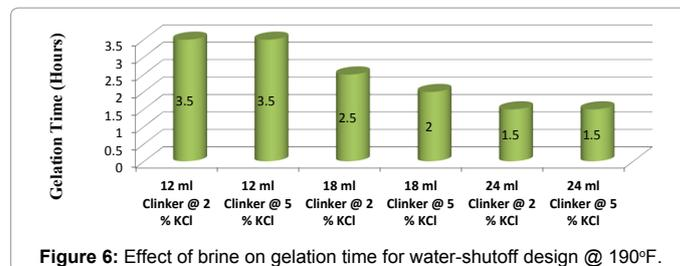
Figure 6: Effect of brine on gelation time for water-shutoff design @ 190°F.
