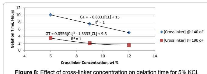
Figure 8: Effect of cross-linker concentration on gelation time for 5% KCl.
