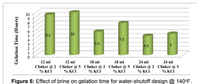
Figure 5: Effect of brine on gelation time for water-shutoff design @ 140°F.
