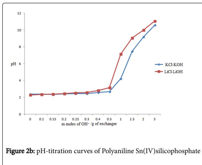
Figure 2b: pH-titration curves of Polyaniline Sn(IV)silicophosphate
