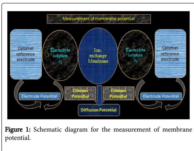
Figure 1: Schematic diagram for the measurement of membrane potential.
