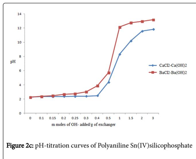
Figure 2c: pH-titration curves of Polyaniline Sn(IV)silicophosphate
