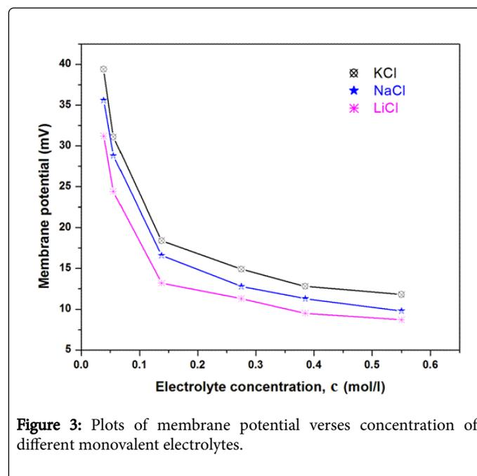
Figure 3: Plots of membrane potential versus concentration of different monovalent electrolytes.
