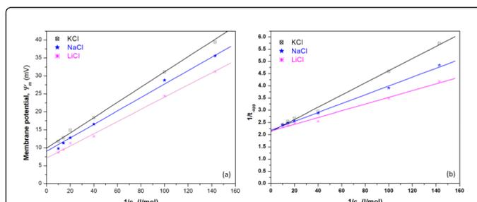
**Figure 4:** Plots of (A) potential values,  $\psi_m$  and (B)  $\frac{1}{t_{app}}$  against  $\frac{1}{c_1}$  of polystyrene based composite membrane for different monovalent electrolytes.
