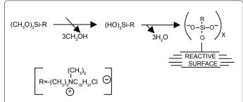
**Figure 1:** Diagram adopted from [23,24] displaying the hydrolysis reaction of Quat-Silsesquioxane on glass surface. Microcidal activity is exerted by the R group exposed at the bound surface.
